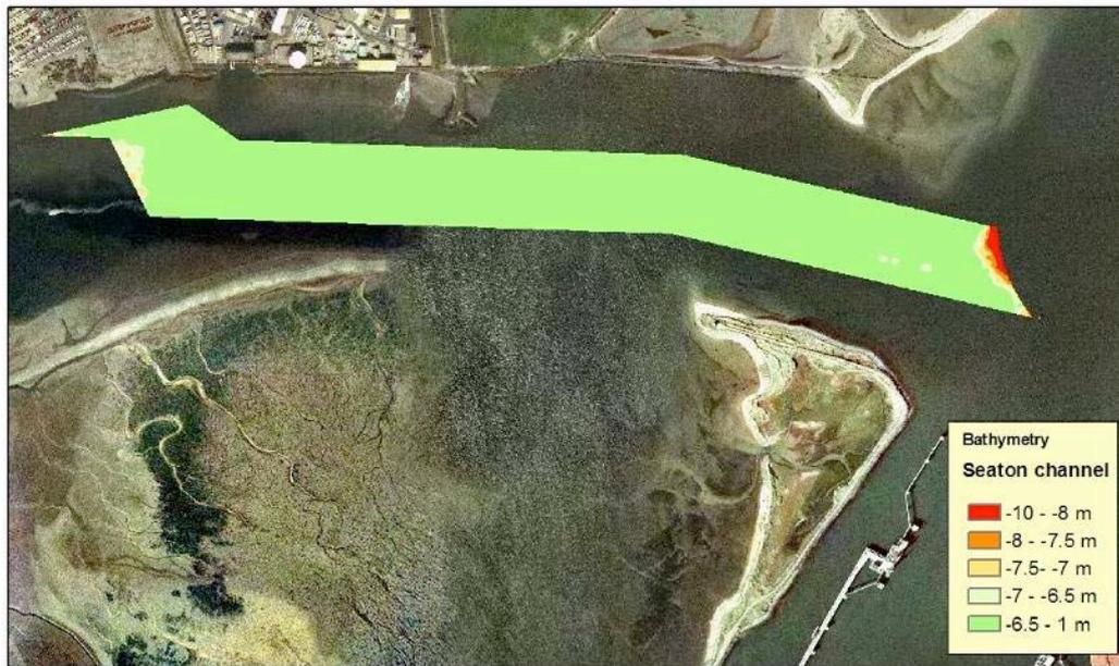
Figure 3-2 Detailed bathymetry for dredging of Seaton Channel
