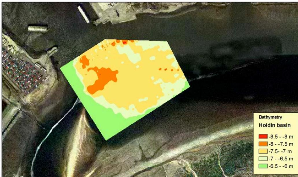
Figure 3-3 Detailed bathymetry for dredging of Holding Basin
