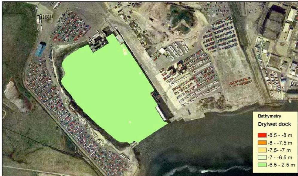
**Figure 3-6 Detailed bathymetry for dredging of Dry/wet dock**
