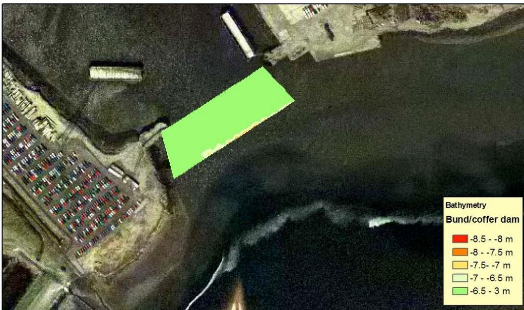
Figure 3-5 Detailed bathymetry for dredging of Bund/cofferdam area
