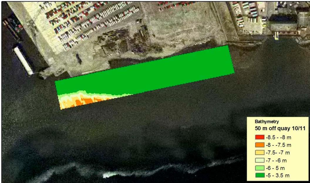
Figure 3-4 Detailed bathymetry for dredging of Quay 10 and 11
