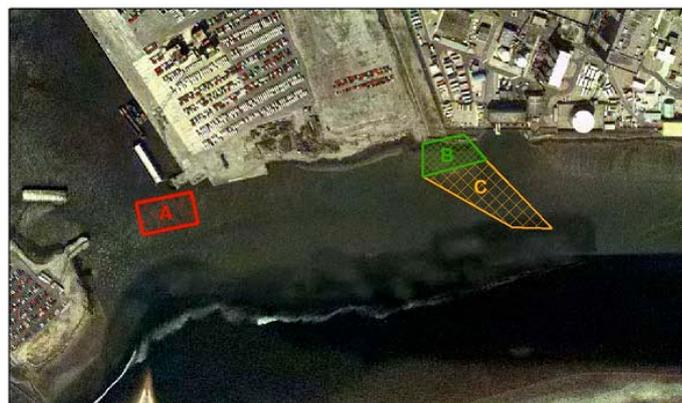
**Figure 3-7 Areas of dredging for the proposed extension of Quay 10 and 11**
